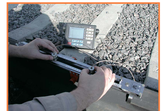
Welding inspection by mirror method using scanner SATS-02R (supplied with)
