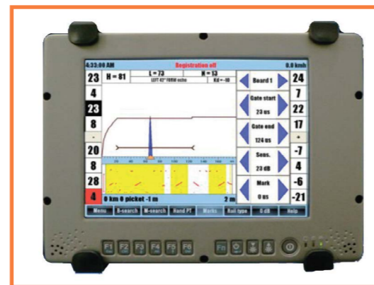
Decision-making of detected defect during inspection period
